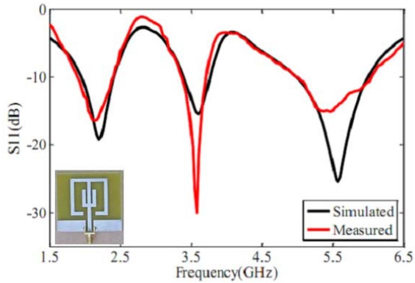
Fig. 1. The simulated and measured reflection coefficient of the antenna.
